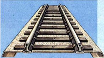
*The new track sections combine the many advantages of the 3-rail system with the realistic appearance of 2-rail track. As in the case of prototype track, the ties are laid on the roadbed and are not part of it. There is therefore no electrical connection between the rails and the roadbed. A parallel circle*
